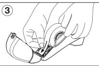
Pull the tape out 30-40mm so that the tip is positioned at the end and the remaining tape rests easily over the row of the rubber bands.
