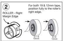
Install the appropriate tape on the roller and place it back into the rail. transparent cover and take out the roller.
