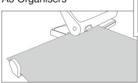
**NOTE:** The cutters nearest the paper guide/ ruler are the only cutters required for A5 punching.
