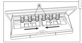
Push the punching cutters A together so the cutter
