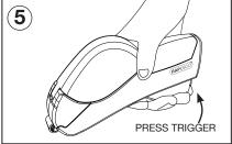
Squeeze the trigger to initialise and load the tape into the front opening.
