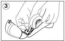
Pull the tape out 30-40mm so that the tip is positioned at the end and the remaining tape rests easily over the row of the rubber bands.
