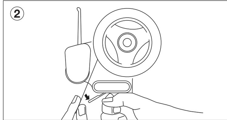
Pull the front end of the tape roll through the slot between the dispenser roller and metal guide. The guide can be held open by pressing down on the extended metal tab. The sticky side of the tape should face down/ away from the edge of the blade. If you have the tape in the wrong way, the tape will stick to the dispenser roller, so make sure the sticky side is face down.
