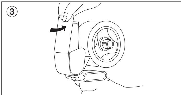
Pull up on the tape so the tape is over the cutting bar/ serrated blade, being careful not to cut yourself on the sharp blade.
