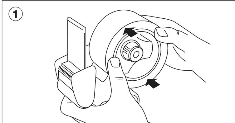
Insert the roll of packing tape onto the large dispenser wheel on the top-right of the tape dispenser with its handle grip to the right. Position the tape roll so that it will unwind with the sticky side facing down as the dispenser is pulled backwards.
