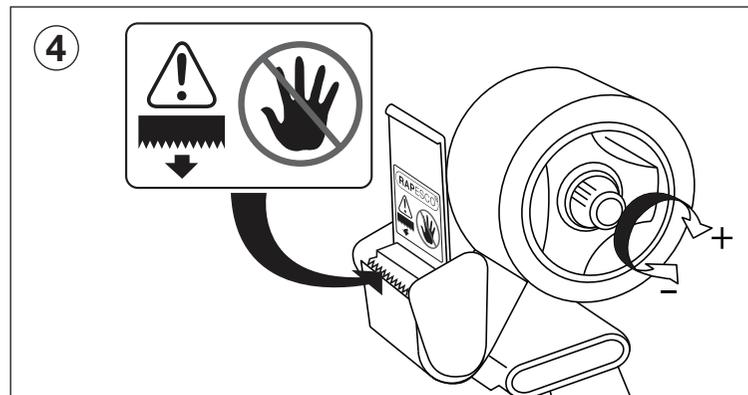
Adjust the tension on the dispenser (in the centre of the large dispenser wheel) to set a smooth and comfortable unwind mechanism.
